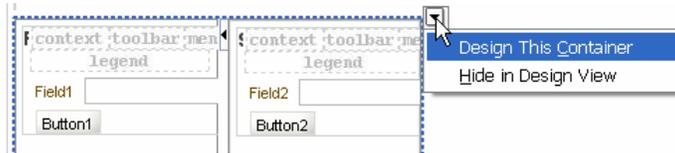
Selecting **Design This Container** opens an editor area that allows you to resize the component borders so that you could achieve a layout such as the following, where all components fit within the panels.
